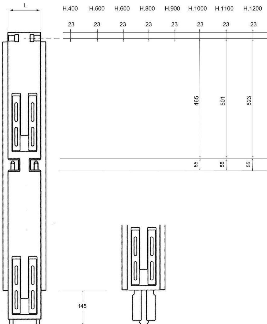
Montanti per apertura universale rovesciabili SP.33mm.Overturning pillars Th.33mm. for tippers
